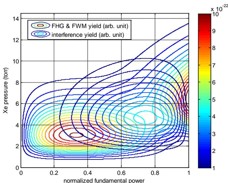
P5I+ P5II /P1+P2 and P5III /P1+P2 for vary with Xe pressure and normalized fundament power at 106.4nm in the tight-focusing limit
